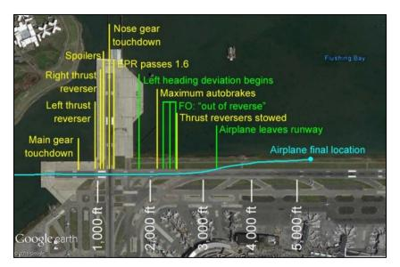
Figure 2: Aircraft ground path (NTSB).
